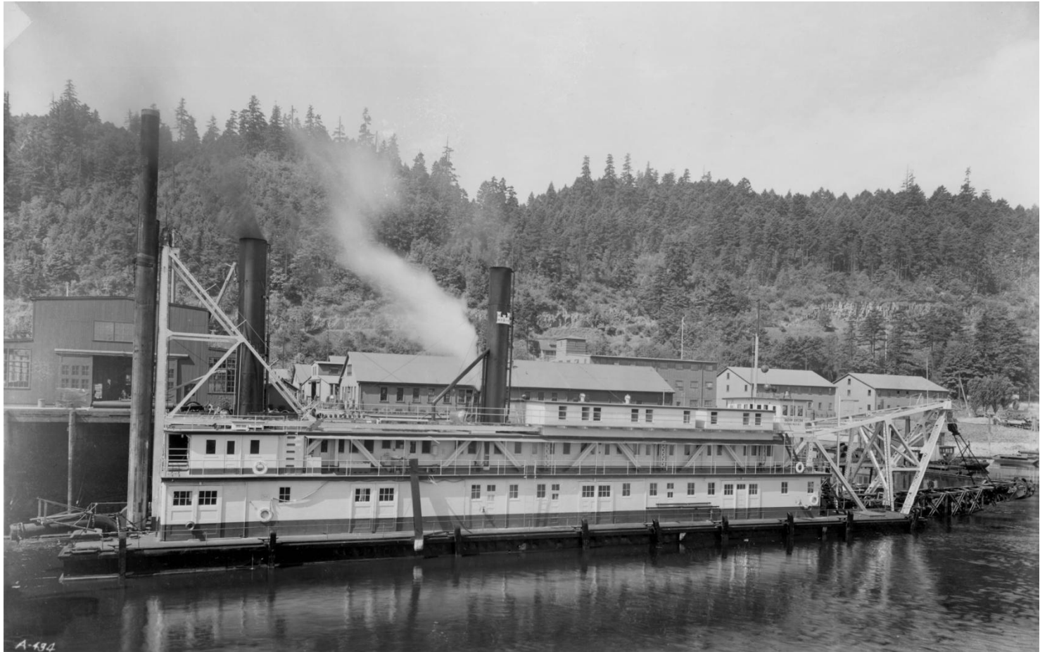
The Portland District, Corps of Engineers, uses the 24-inch hydraulic pipeline dredge Wahkiakum for work on the Willamette and Columbia Rivers in Oregon. Non-propelled, she has a steel hull with a length of 194 feet. Her beam is 38 feet. She was built in 1913 by Portland Iron Works. She has a crew of 52 men.
